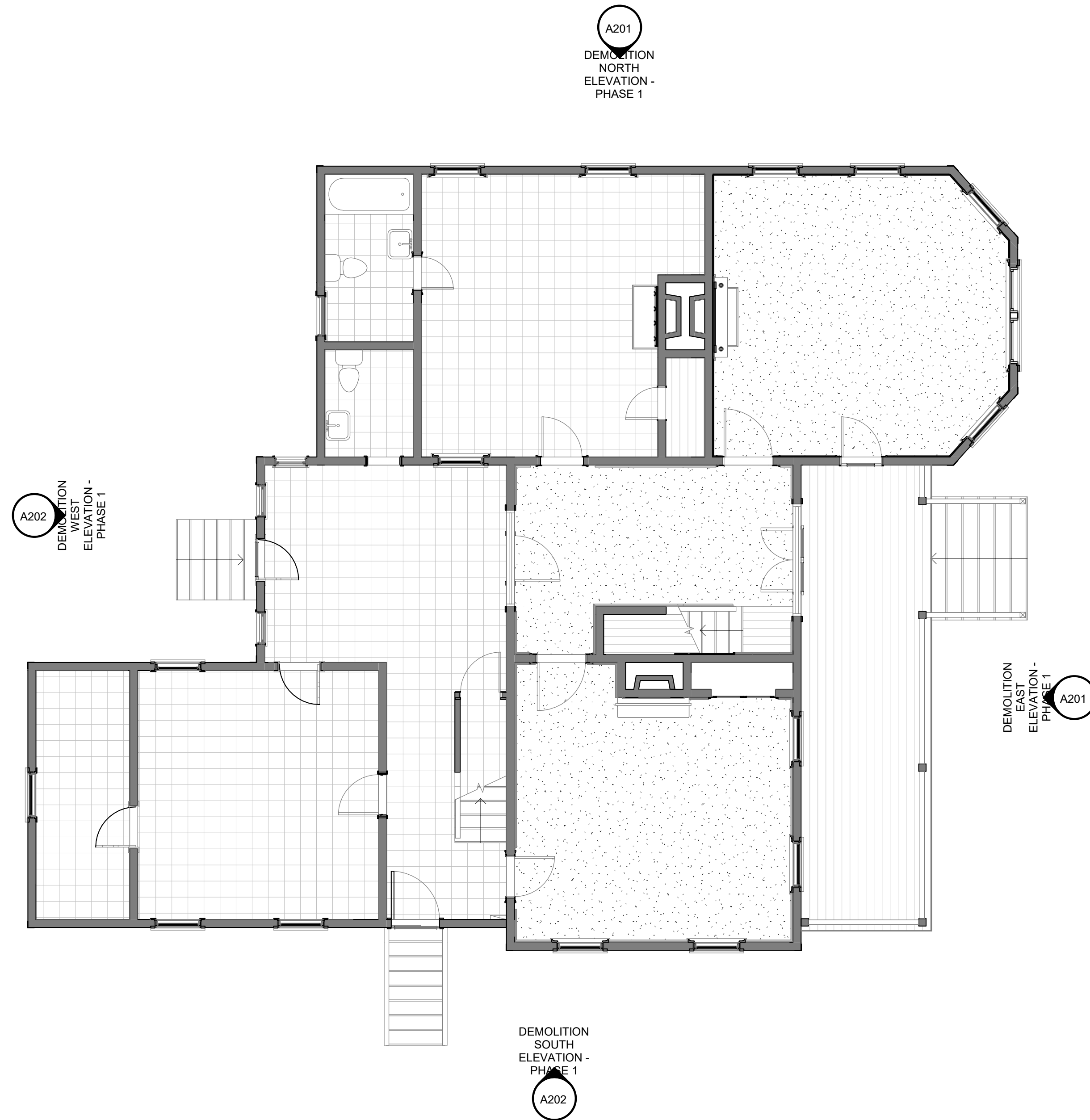
1 01 - DEMOLITION 1ST FLR PLAN - PHASE 1 3/16" = 1'-0"
