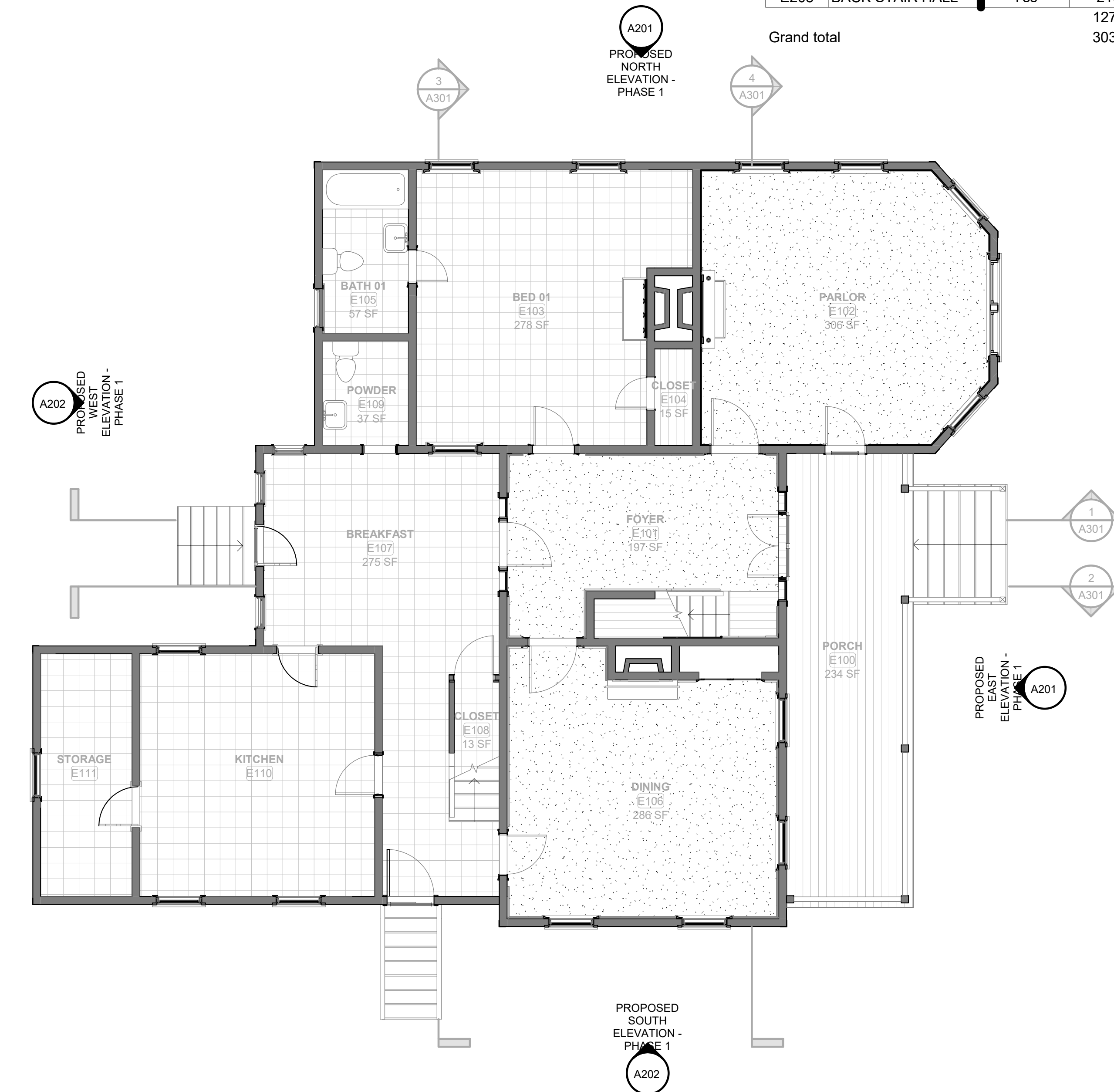
2 01 - PROPOSED 1ST FLR DIMENSION PLAN - PHASE 1 3/16" = 1'-0"
