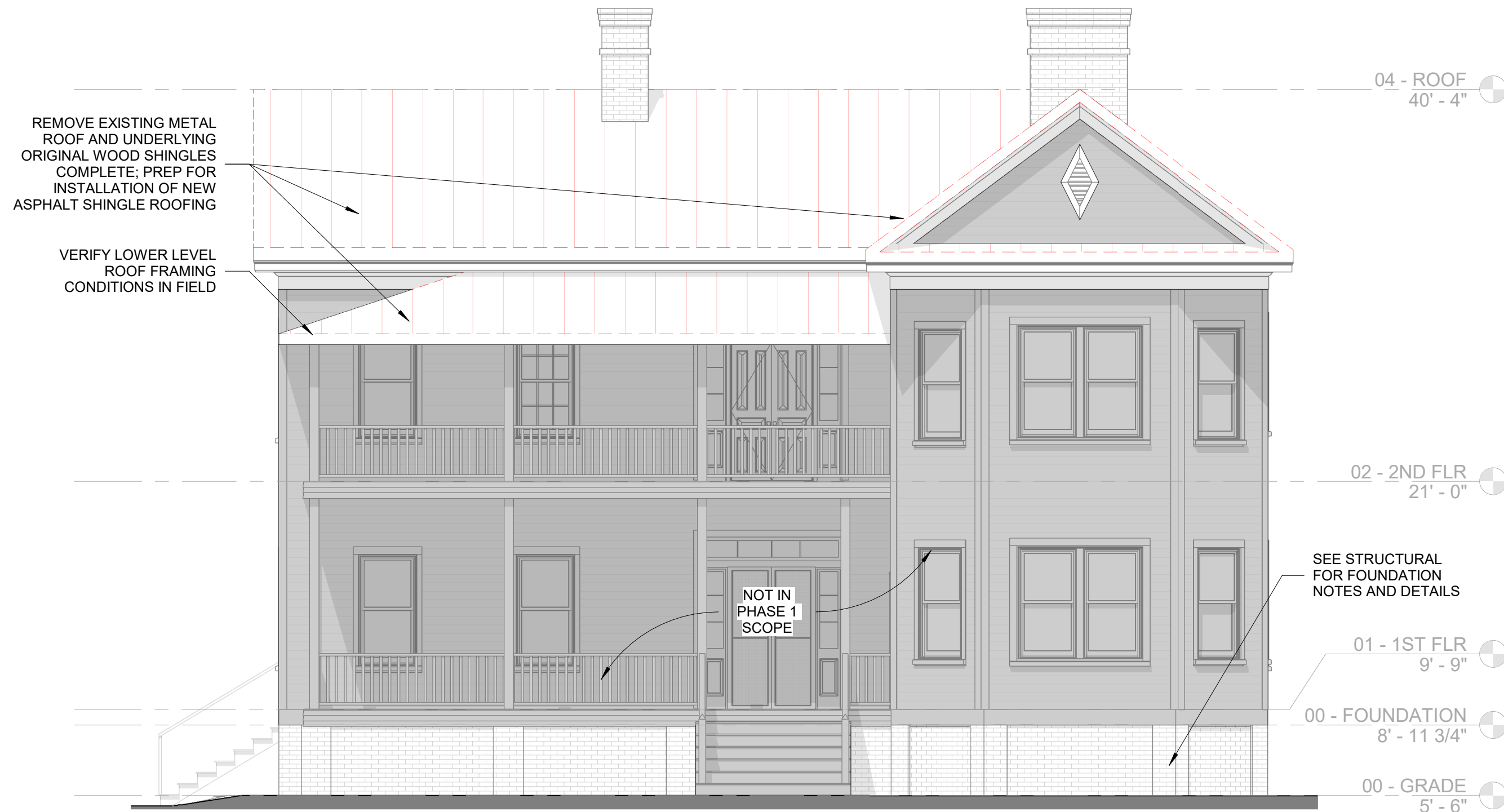
① DEMOLITION EAST ELEVATION - PHASE 1 3/16" = 1'-0"
