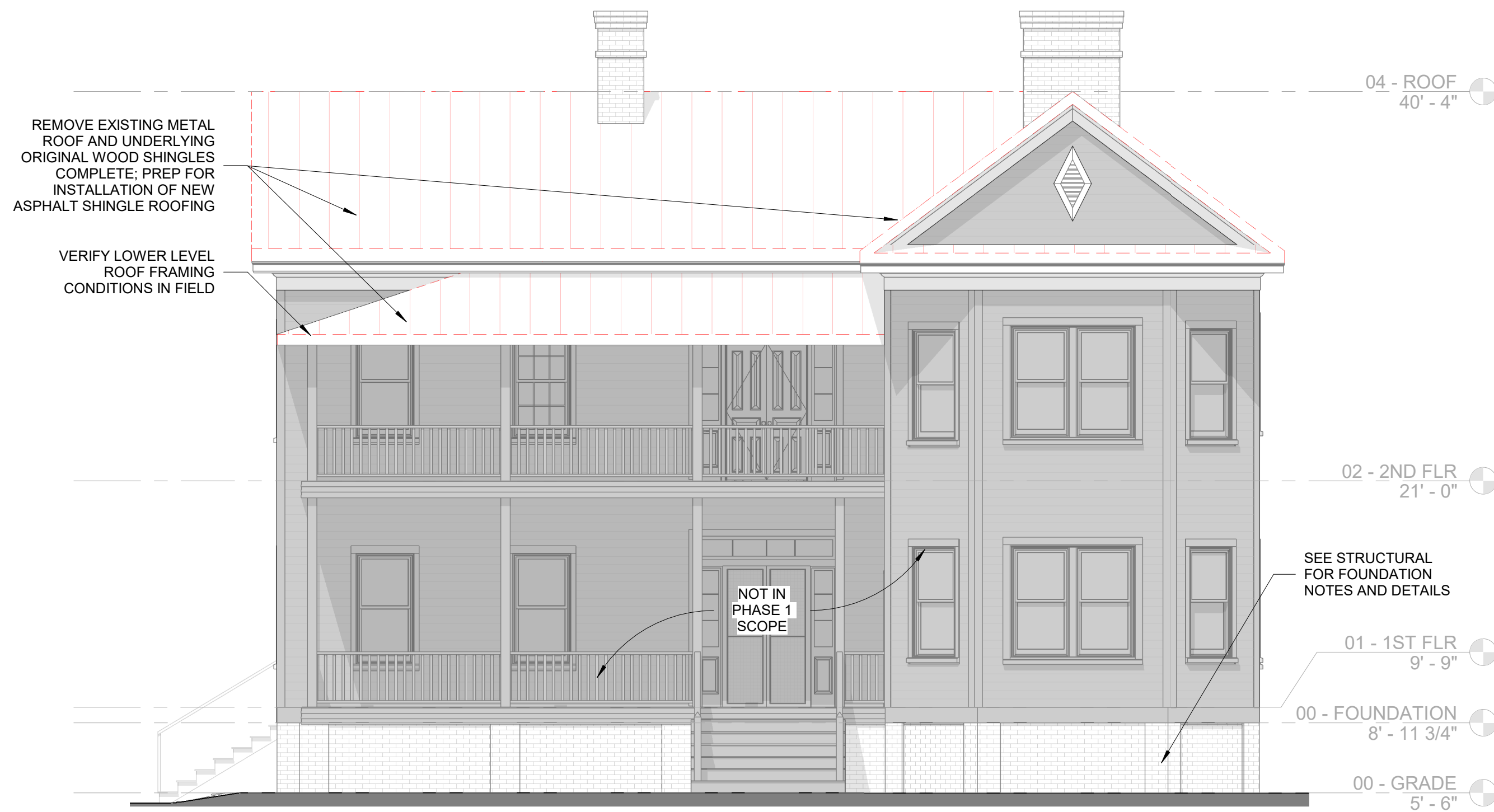
① DEMOLITION EAST ELEVATION - PHASE 1 3/16" = 1'-0"
